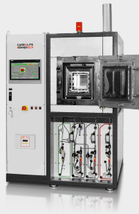
HTK 8 MO/16-1G automatic up to 1600°C with optional hydrogen equipment
