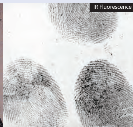
US $20 banknote dusted with fpNATURAL® 2 , illuminated in the near-IR and examined at 850nm
