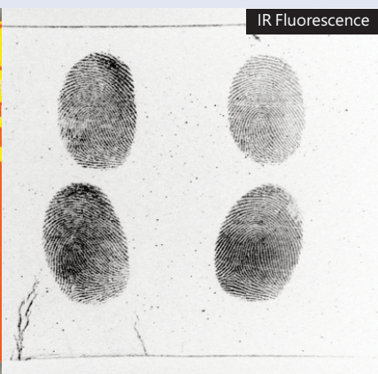
Glossy card packaging dusted with fpNATURAL® 2 , illuminated in the near IR (780-nm) and examined at 850nm
