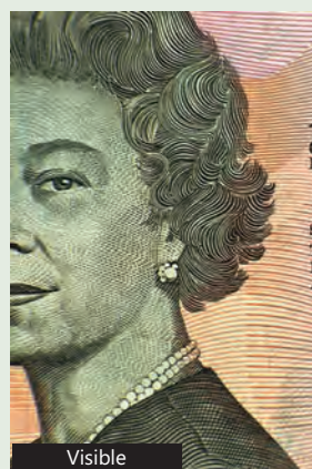
AUD $5 Polymer banknote dusted with fpNATURAL® 1 , illuminated with red light and examined at 780nm
