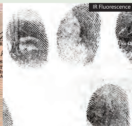
AUD $5 Polymer banknote dusted with fpNATURAL® 1 , illuminated with red light and examined at 780nm
