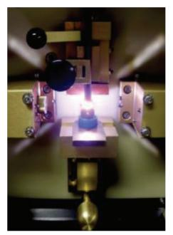
Figure 3: RDE Spectrometer Sample Stand Showing Oil Sample Being "Burned"
