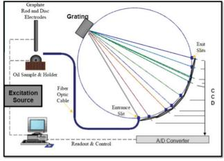
Figure 4: Schematic of a Rotating Disc Electrode Optical Emission Spectrometer for Oil Analysis
