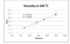
Figure 10. Comparison of Viscosity measurements between MicroLab and Lab D445 for a series of fresh Shell Omala oils with grade from ISO46 to ISO 320..
