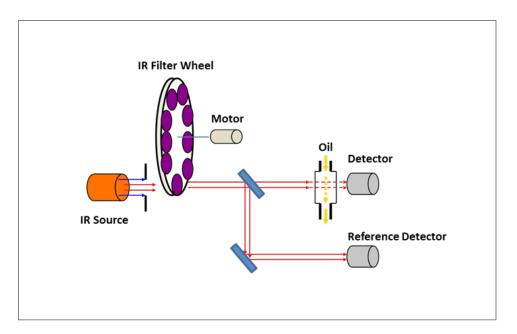
nitration peak around 1650 cm<sup>-1</sup> becomes significantly more intense as an engine oil is sampled over a specified time, then nitration has occurred which may indicate improper air/ fuel ratio. Total Base Number can be monitored by the TBN additive depletion which appears as a decrease in the absorbance peaks in the region of 1000 to 1900 cm<sup>-1</sup>. Water that is dissolved in oil shows a characteristic absorption peak between 3200 and 3800 cm<sup>-1</sup>.
