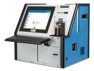
The MicroLab is the ideal trending tool to allow companies to identify mechanical problems before they become catastrophic equipment failures. The ability to track the serviceable life of the oil to know when they can safely extend the oil drain interval helps save money on oil consumption, oil disposal and labor costs associated with unnecessary oil drains.
