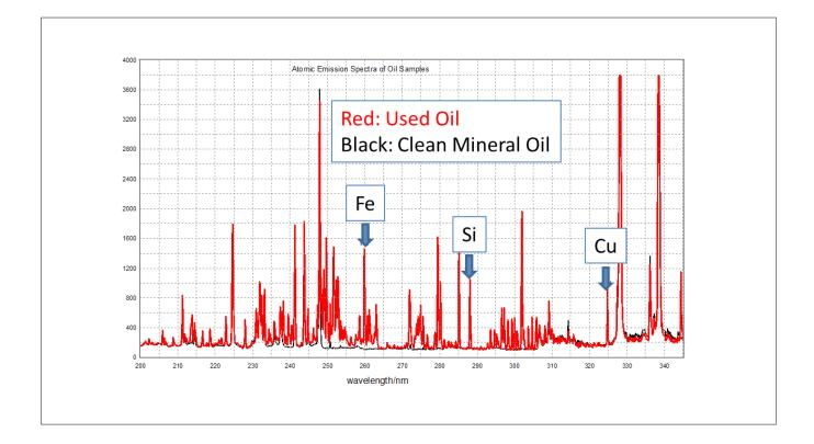
Figure 3. Representative emission spectra from two oil samples: the spectrum in red is from a customer used oil sample and the one in black is white mineral oil shown here for comparison. each element and comparing to the peak area of the standard samples measured at the time of instrument calibration during production, the concentration (in ppm) of the element is then determined.
