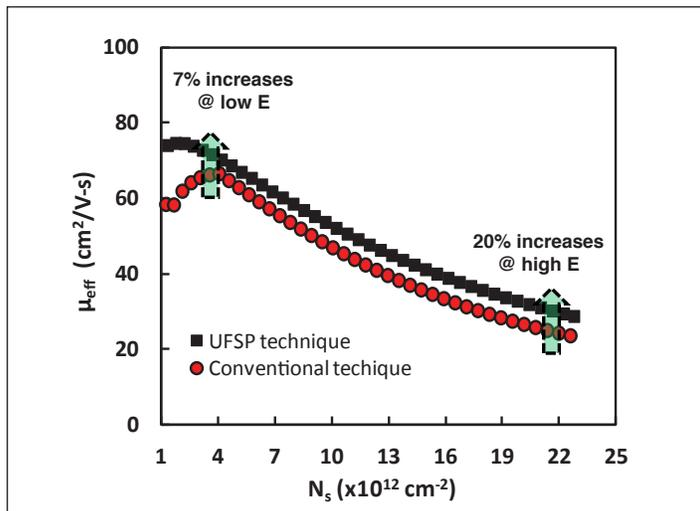
**Figure 9. A comparison of mobility extracted by UFSP and conventional technique for a device with  $HfO_2/SiON$  dielectric of considerable fast trapping.**
