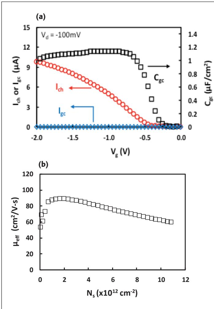
Figure 6. (a)  $I_{\text{ch}}$ ,  $I_g$ , and  $C_{\text{gc}}$  extracted simultaneously from the currents in Figure 5 by using Equations (2)–(5). (b) Channel effective mobility extracted from  $I_{\text{ch}}$  and  $C_{\text{gc}}$  from (a).
