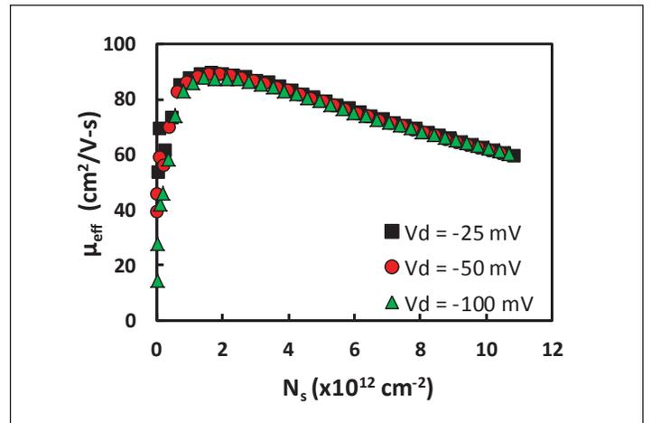
Figure 7. The effective channel mobility,  $\mu_{\text{eff}}$  extracted under three different  $V_d$  by using UFSP technique.
