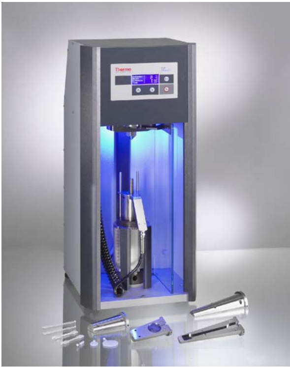
Fig. 3: HAAKE MiniLab Pro and moulds
