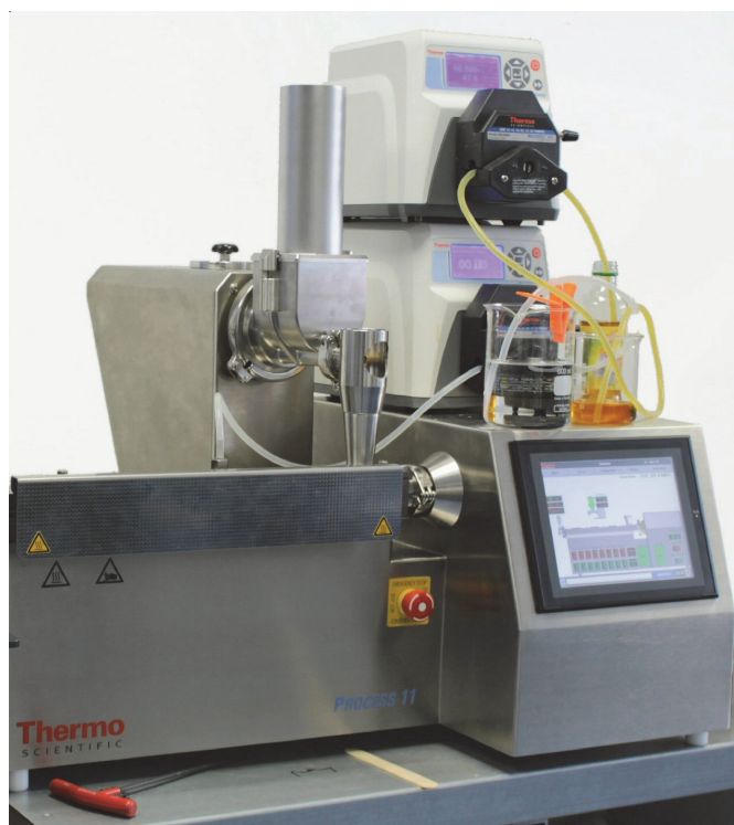
Fig 1: Feeding powders and liquid ingredients into the extruder.
