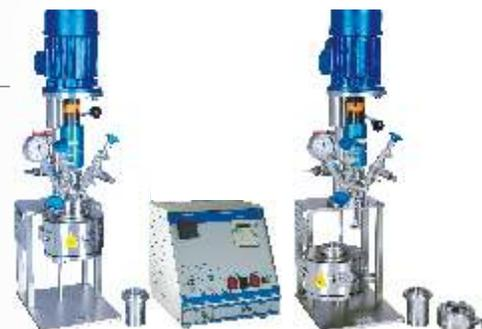
50 ml & 100 ml interchangeable reactors with fixed head design
