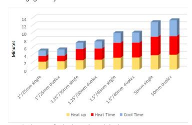
Fast Cycle times for both single and duplex mounts \*Cycle times are typical actual times may be faster or slower depending on media used, sample type/size, water temperature, and other factors.
