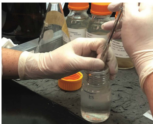
4 Technician filtering sample through solid phase extraction disk per EPA Method 1664B
