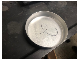
6 Oil and grease residue after evaporation in fume hood
