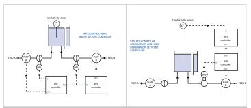
Fig 1: Ratio control of two flows
