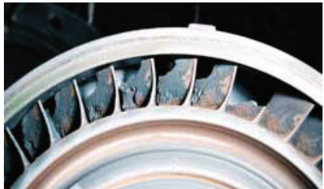
Figure 4: Severe sulfidation corrosion on turbine blades leads to lost efficiency and blade failure.
