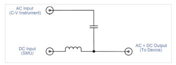
Figure 1: Typical Bias Tee Block Diagram
