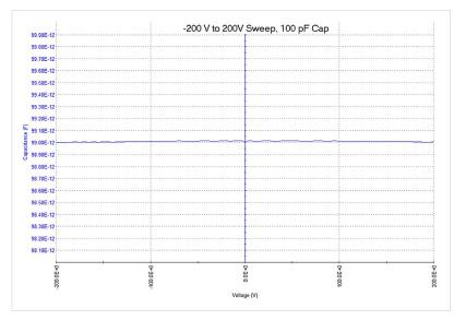
Figure 14: ±200 V Sweep on 100 pF Capacitor
