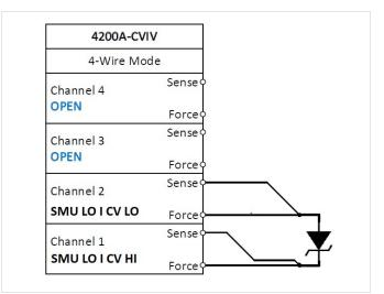
Figure 2: High Voltage C-V Connections for Zener Diode using the  $\ensuremath{\mathsf{CVIV}}$
