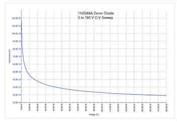
Figure 12: Results of C-V Sweep of Zener Diode
