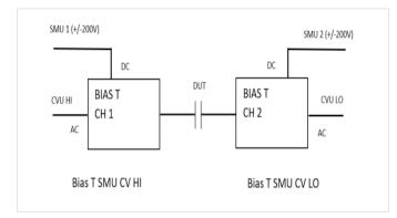
Figure 5: BiasT SMU CV HI or LO Channel Configuration
